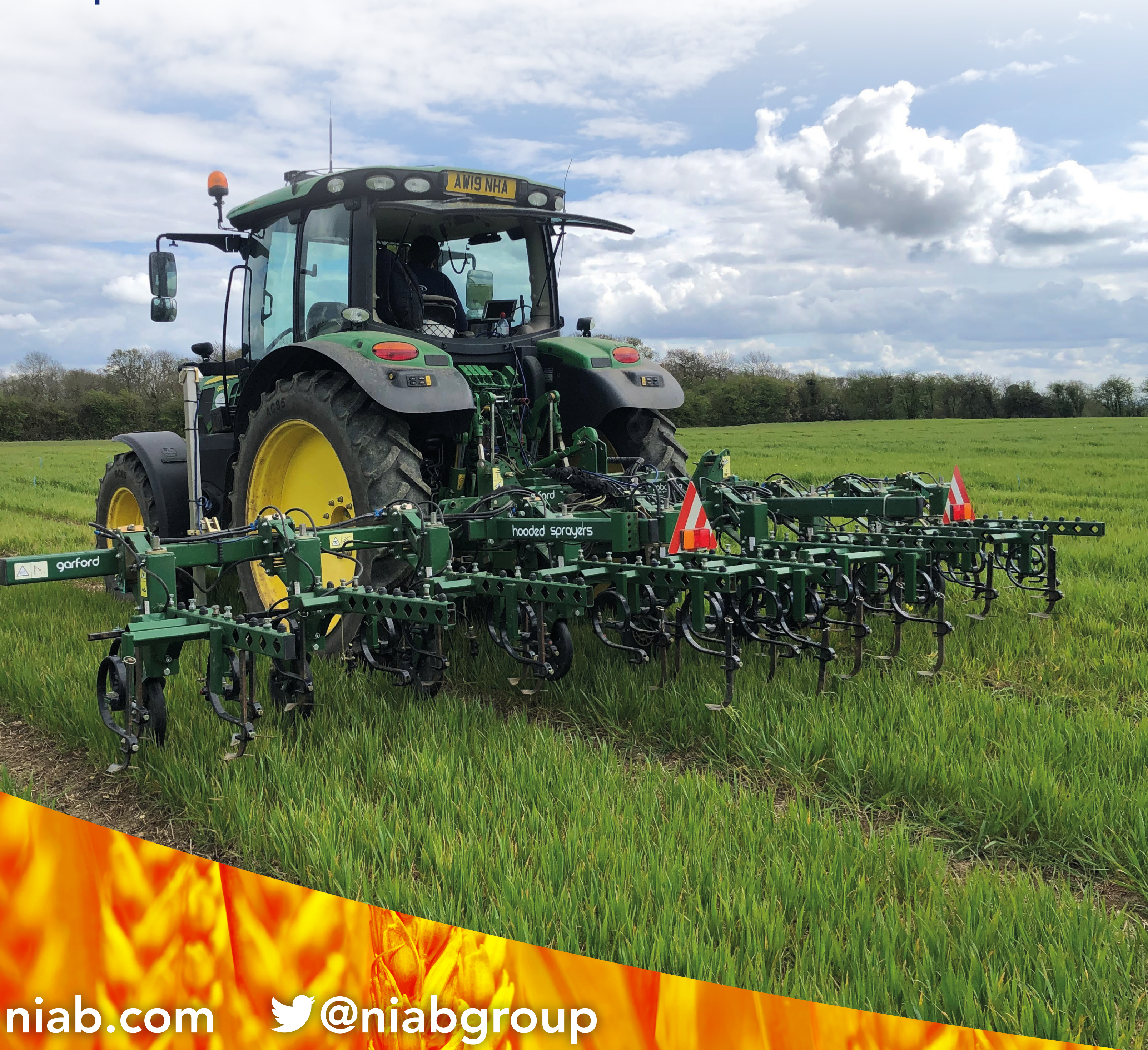
Figure 1. The Garford Robocrop set up for inter-row cultivation
