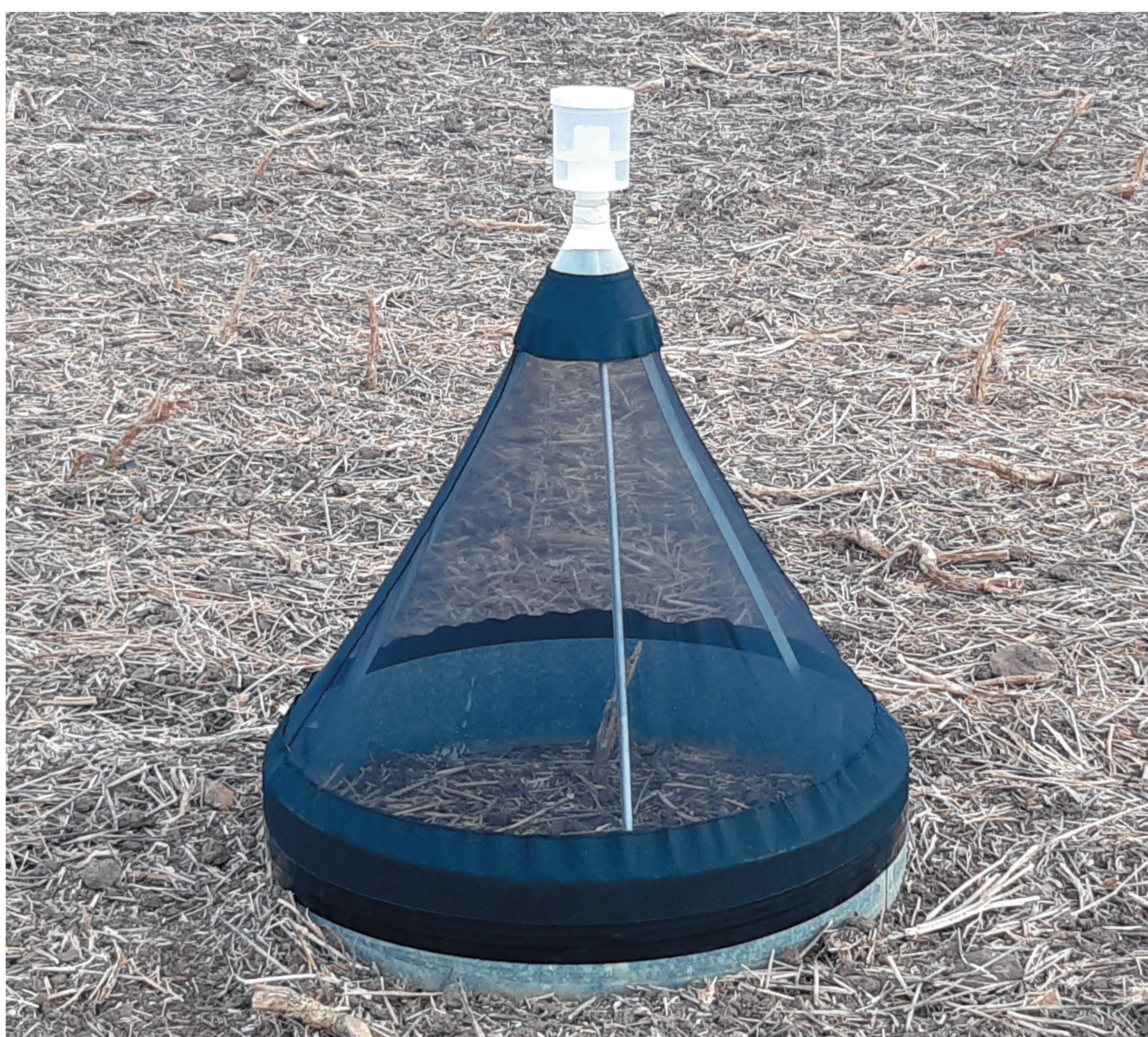
Figure 1. Insect emergence trap, developed by Rothamsted Research
